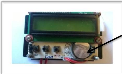
Open the top cover locate the Battery placed below LCD
