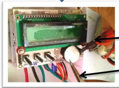
Press the battery lock with the help of a small screw driver and pluck out the battery with the help if a pointed object or tweezers
